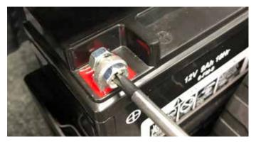
Securely tighten the positive (+) battery cable (red boot) to the positive (+) battery post. Make sure boot is over battery post.
