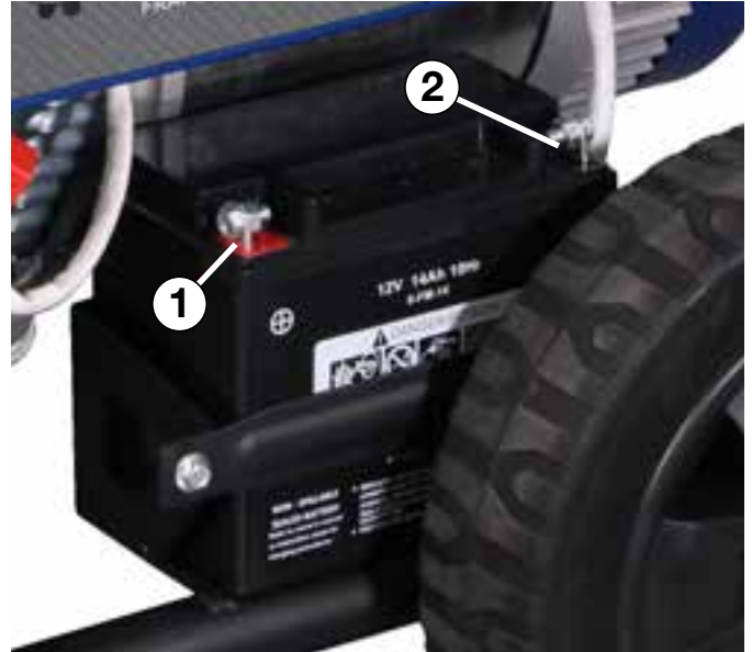
Figure 6 - Attaching the Negative (-) Battery Wire (black)
