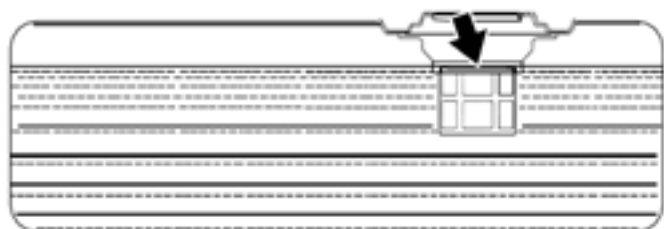
Figure 12 - Maximum Gasoline Fill Level
