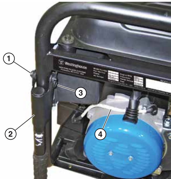
Figure 7 – Attaching the Handles
