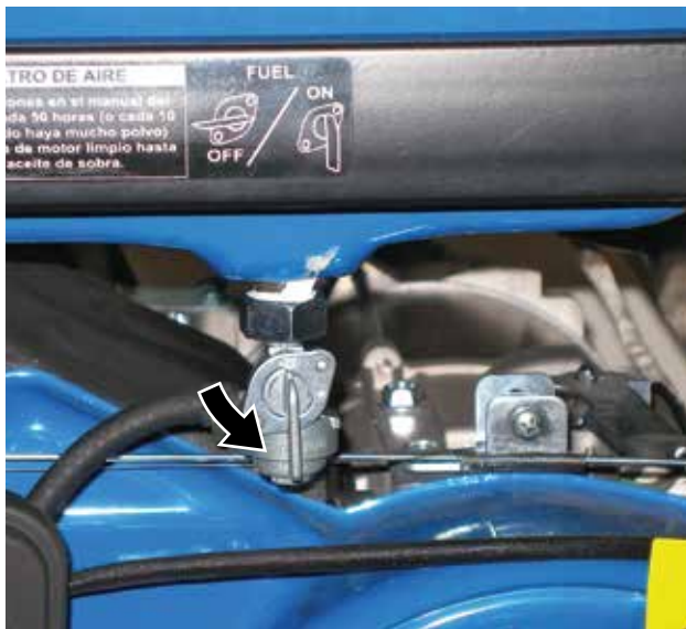
Figure 22 – Fuel Shutoff Valve in the ON Position
