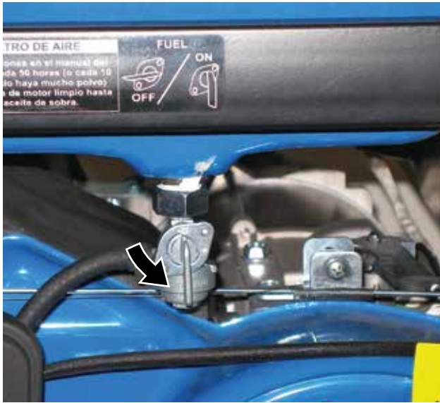
Figure 17 – Fuel Shutoff Valve in the ON Position
