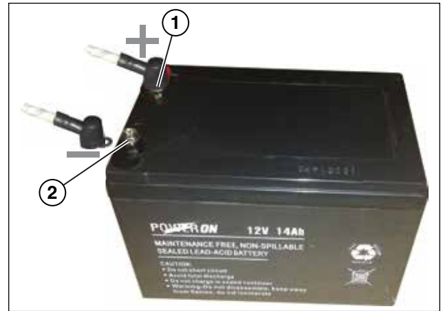
Figure 8 – Attaching the Negative (-) Battery Cable (Black)
