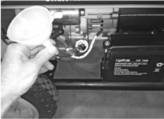
Figure 28 – Adding Engine Oil
