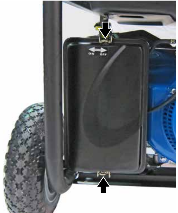
Figure 35 – Installation of Air Filter Cover
