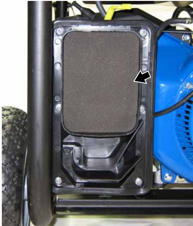
Figure 32 – Removing Fine Inside Air Filter
