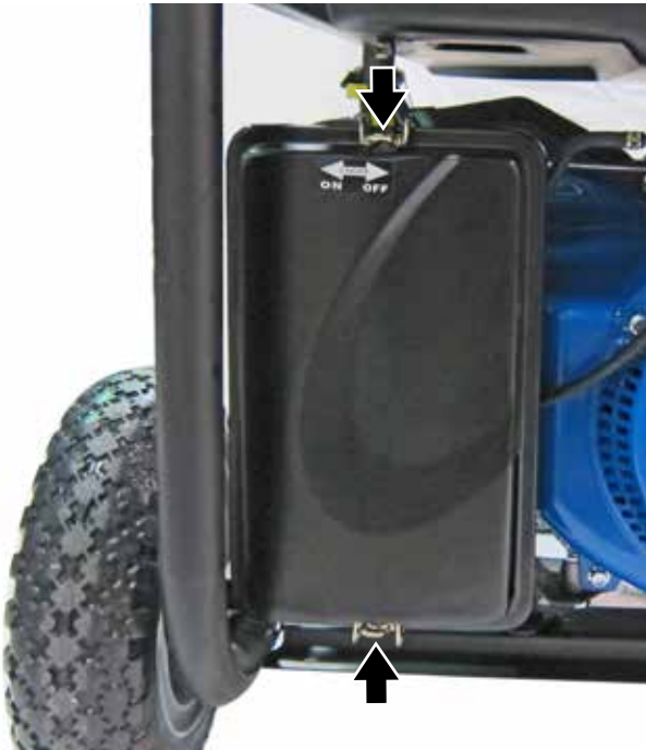
Figure 30 – Removing Air Filter Cover
