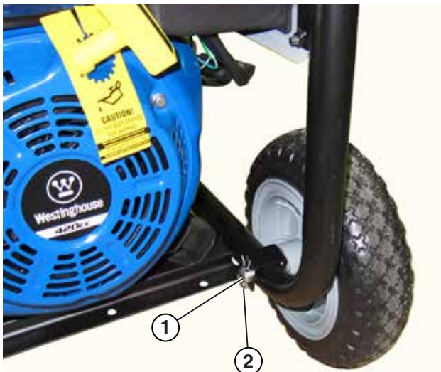
Figure 6 – Assemble Wheels to Frame
