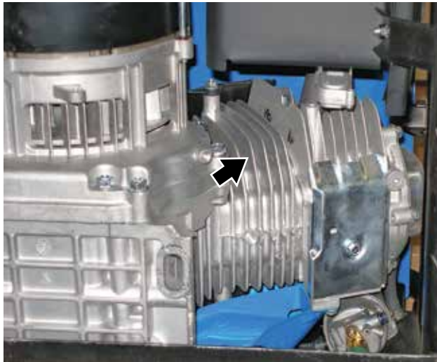
Figure 44 – Engine Cooling Fins
