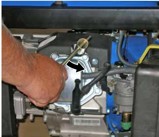
Figure 37 – Removing Spark Plug
