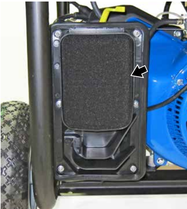
Figure 31 – Removing Coarse Outside Air Filter
