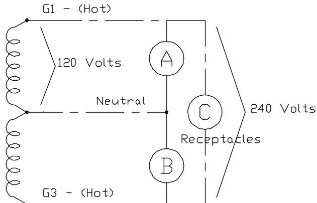
Check the appliance or tool nameplates for the current and voltage to insure compatibility. Remember that power taken from receptacle C reduces the power available at both A and B. Any remaining 120 volt loads should be equally divided between A and B. Failure to split the load will cause permanent damage to the stator. Although circuit breakers are provided, damage due to overloading constitutes abuse and will not be warranted. Refer to the generator nameplate for your unit's capabilities.
