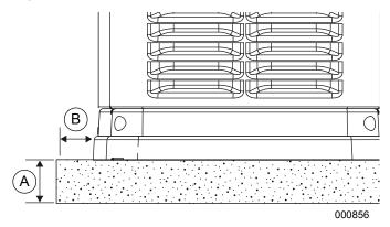
Figure 3-3. Compacted Soil or Gravel Pad
