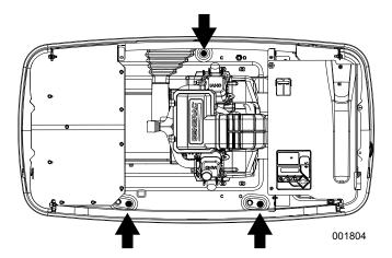
Figure 4-2. Mounting Hole Locations
