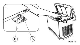
Figure 2-8. Generator Main Line Circuit Breaker
