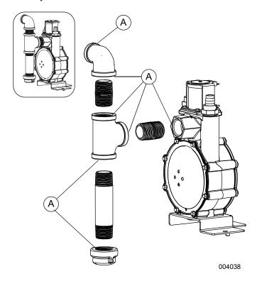
Figure 5-5. Connection Points to Leak Check
