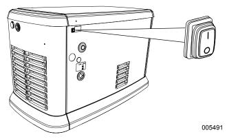
Figure 2-10. Auxiliary Shutdown Switch (all models)
