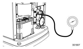
Figure 5-4. Checking Pressure with Manometer
