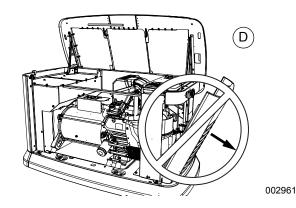
Figure 2-5. Intake Side Panel Removal
