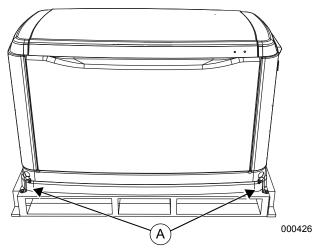
Figure 2-3. Generator on Pallet
