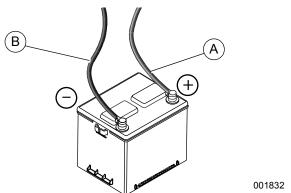
Figure 6-2. Battery Cable Connections
