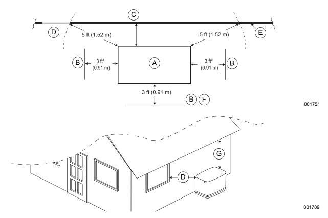
Figure 3-1. Installation Clearances
