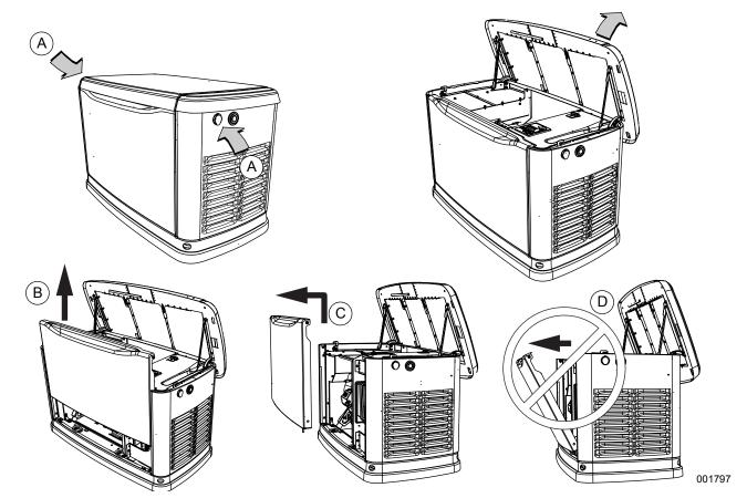
Figure 2-4. Side Lock Location and Front Panel Removal
