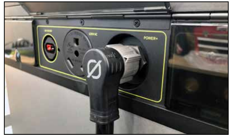
The Flying Leads to Power+ Cable plugs into the back of the Yeti PRO at a 90-degree angle for more compact cabling.
