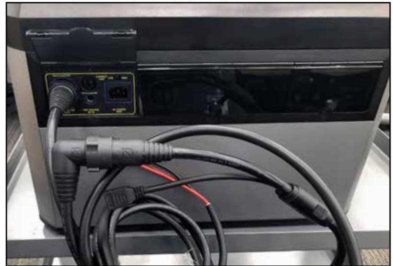
Escape Remote Display HPP+ Power and Data Adapter plugged into Yeti, and HPP+ to Flying Leads Cable plugged into the Power and Data Adapter.
