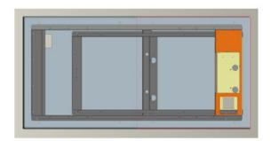
While the GenPad LC is made specifically to fit the frame of 32-60kW gas generators, it can also readily accommodate the smaller frame of 22-30kW units.
