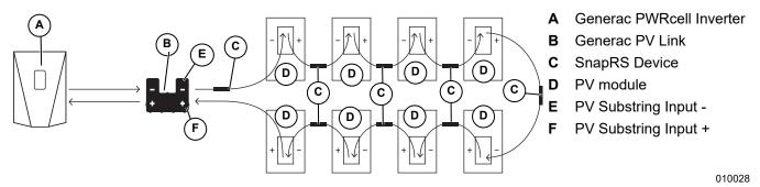
Figure 3-1. Single-String PV Array with Generac SnapRS™ Devices
