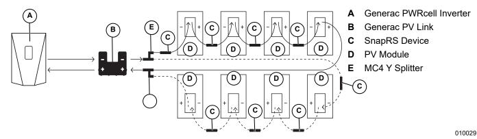
Figure 3-2. Parallel-Input PV Array with Generac SnapRS™ Devices
