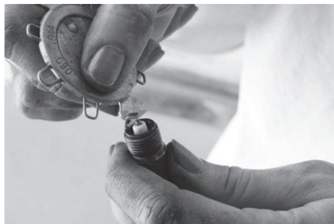
Figure 5-17. Adjust Spark Plug Gap
