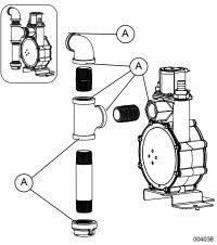
Figure 5-5. Connection Points to Leak Check
