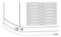
Figure 4-1. Installing Base Plugs
