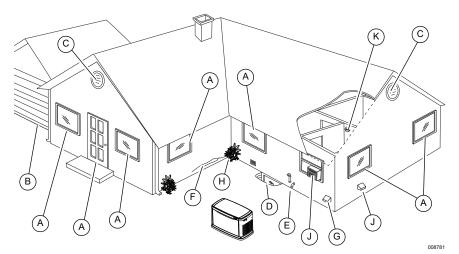
Figure 3-1. Carbon Monoxide—Potential Entry Points
