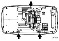
Figure 4-2. Mounting Hole Locations
