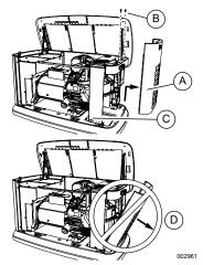
Figure 2-6. Intake Side Panel Removal
