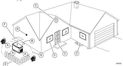
Figure 3-2. Generator Distance Requirements
