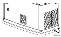
Figure 4-1. Integrated Composite Pad
