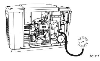
Figure 5-4. Checking Pressure with Manometer
