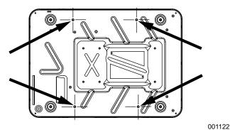
Figure 4-2. Mounting Hole Location
