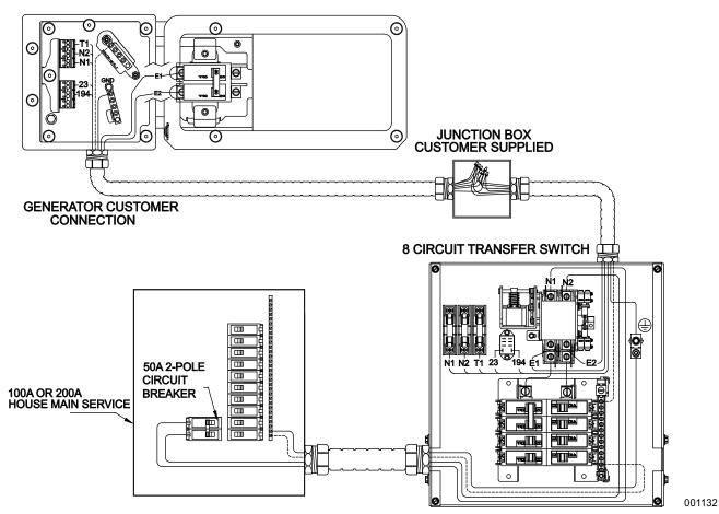
Figure 6-2. Main AC Wiring
