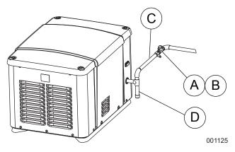
Figure 5-3. Gas Line Connections
