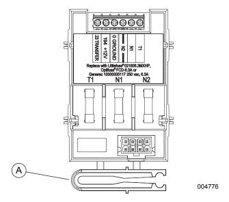
Figure 4-2. Fuse Removal and Installation Tool
