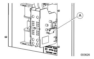
Figure 3-3. Auxiliary Contact
