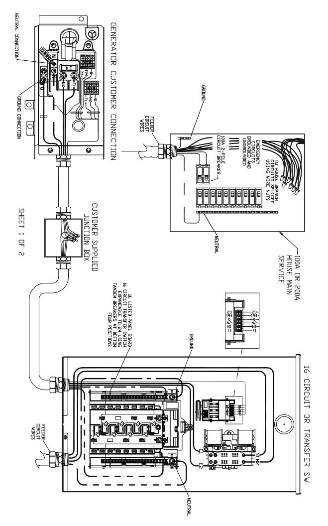
EXPLODED VIEW: INTERCONNECTION DIAGRAM 3R 16 CIRCUIT DRAWING #: 10000016945
