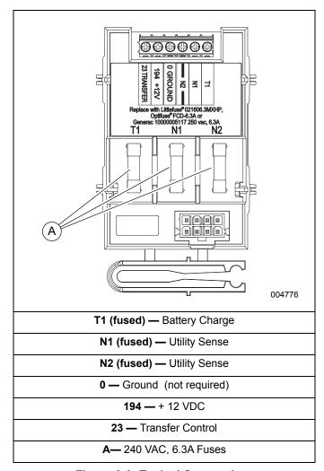
Figure 3-2. Typical Connections
