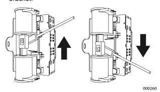
Figure 4-1. Manual Transfer Switch Operation
