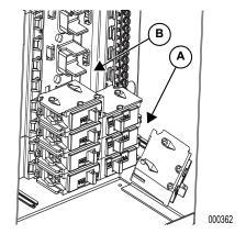
Figure 3-1. Installing Breakers
