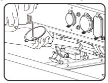
5.Replace oil fill cap/dipstick and fully tighten. 6.Oil level should be checked prior to each use or at least every 8 hours of operation. Keep oil level maintained.
