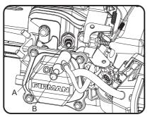
A- Spark plug B- Spark plug cap
