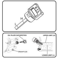
4.Using oil funnel, slowly pour contents of provided oil bottle into oil fill opening to the "H" mark on dipstick. Be careful do not overfill. Overfilling with oil could cause the engine to not start or hard starting.
