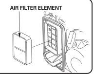
(b) After wetting the element with clean engine oil squeeze it tight by hand.
