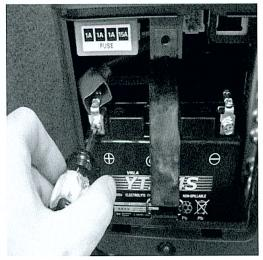
4. After the grommet is installed, loosen the screw on the positive battery terminal using a Phillips screwdriver, then snap the fork terminal from the red receiver wire into place and tighten holding screw. Repeat for the negative battery terminal using the black receiver wire.
