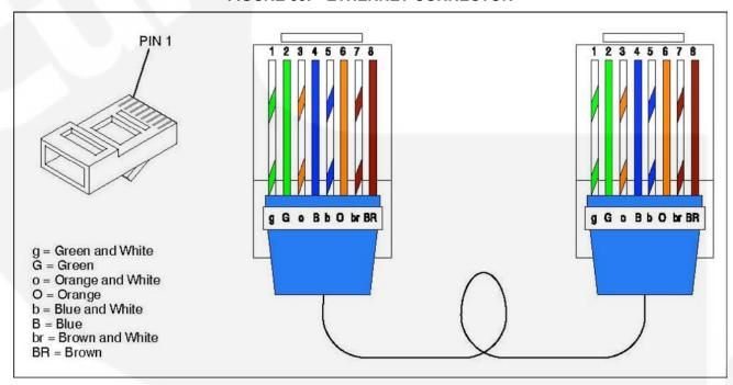
FIGURE 40. ETHERNET RJ-45 CONNECTOR WIRING
