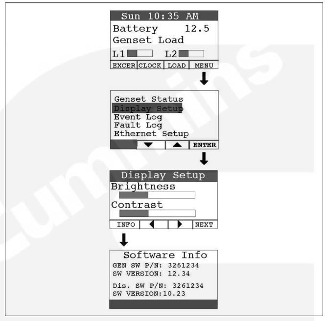
FIGURE 19. DISPLAY SETUP AND SOFTWARE INFO SCREENS
