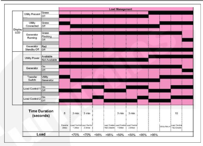
FIGURE 7. LOAD MANAGEMENT TIMING DIAGRAM
