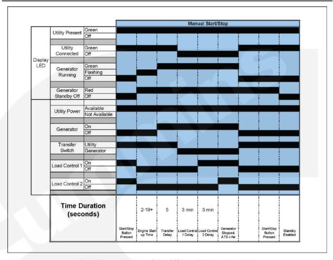
FIGURE 6. MANUAL START/STOP TIMING DIAGRAM
