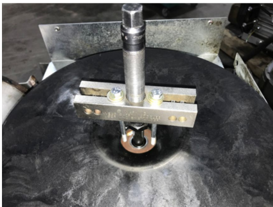
FIGURE 64. PULLING FAN HUB OFF ROTOR
