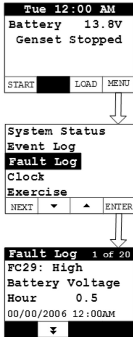
FIGURE 11. FAULT LOG SCREEN
