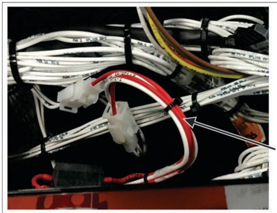
FIGURE 6. ROUTING OF THE EMERGENCY STOP CONTACT BLOCK WIRES (GENERATOR SETS WITH A DISPLAY PANEL RUBBER PLUG ONLY)
