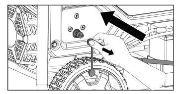
Connect the other end of the LPG hose to the LPG cylinder valve and hand tighten.
