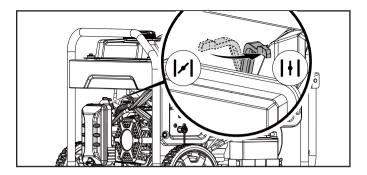
9. Press and hold the ignition switch in the "START" position for up to 5 seconds or until started.
