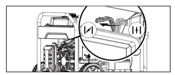
Press the ignition switch to the "START" position for 2-3 seconds.
