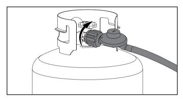
5. Open valve on LPG cylinder and check all connections for leaks by wetting the fittings with a solution of soap and water. Bubbles which appear or bubbles which grow indicate that a leak exists. If a leak exists at a fitting then turn off the valve on the cylinder and tighten the fitting. Turn the valve back on and recheck the fitting with the soap and water solution. If the leak continues or if the leak is not at a fitting then do not use the generator and contact customer service.
