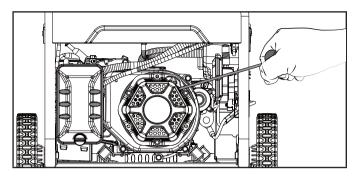
8. Move the choke lever to the "RUN" position.
