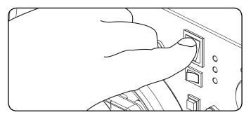
ELECTRIC START: Press and hold the ignition switch to the "START" position. Release as the engine begins to roll over. If the engine fails to start Electric and Recoil Start Cont'd.
