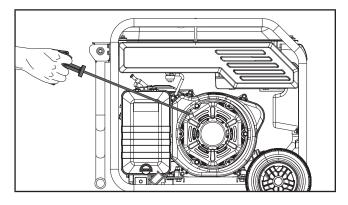
Once engine starts, push choke button to the "RUN" position.
