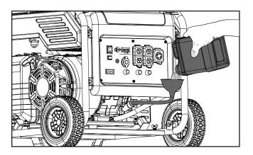
4. Check engine oil level at every use and add as needed.
