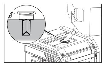
Fuel gauge on top of tank will read "F" when full of gasoline and "E" when tank is empty and needs to be refilled.
