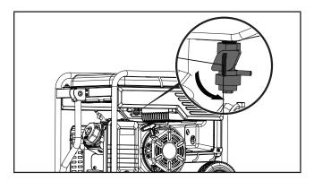
4. Push the engine switch to the "ON" position.
