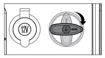
5. Pull choke knob out to the "CHOKE" position.
