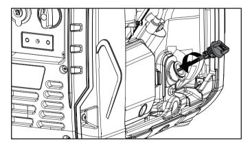
Tilt the generator on its side and allow the oil to drain completely.
