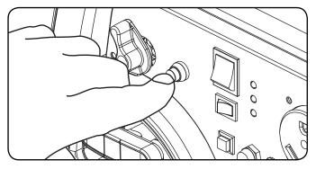
6. Turn the ignition switch to the "On" position.
