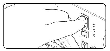
7. ELECTRIC START: Press and hold the ignition switch to the "START" position. Release as the engine begins to roll over. If the engine fails to start Electric and Recoil Start Cont'd.
