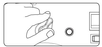
4. Turn the battery switch to the "On" position.
