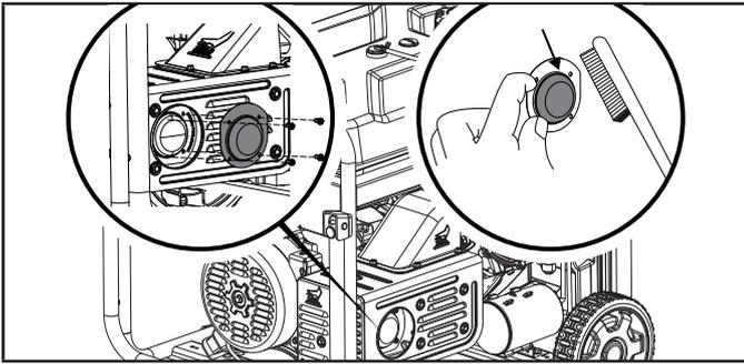
5. Replace the spark arrestor if it is damaged.
