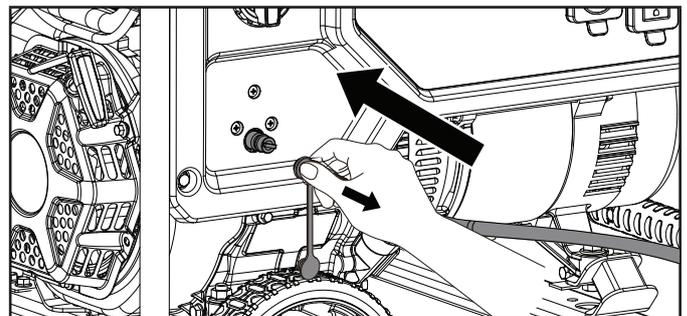
4. Connect the other end of the LPG hose to the LPG cylinder valve and hand tighten.
