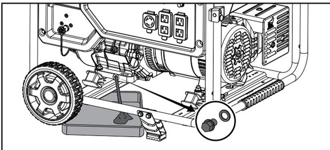
3. Replace the oil drain bolt.
