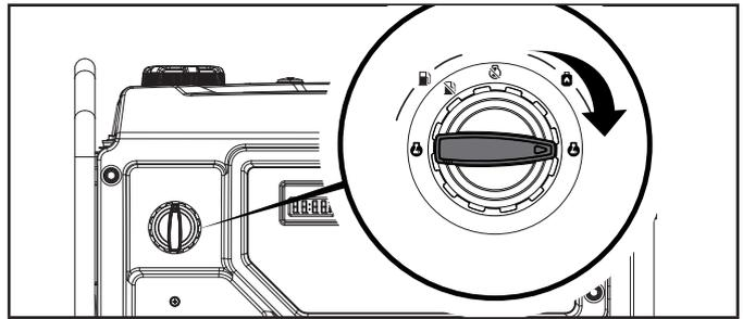
6. Move the choke lever to the “CHOKE” position.
