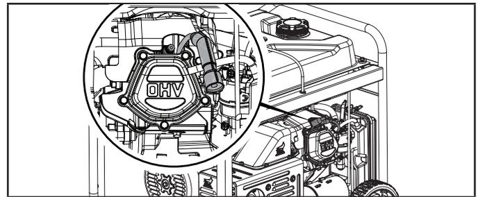
3. Inspect the electrode on the plug. It must be clean and not worn to produce the spark required for ignition.
