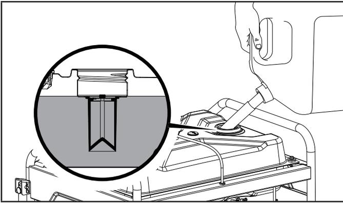
3. The approximate fuel level is shown on the fuel gauge on top of the fuel tank.
