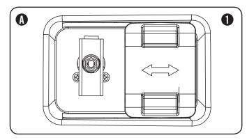
Once a fuel source has been selected, the user must turn the fuel valve to the vertical position to open the fuel valve. (1)
