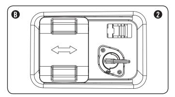
To turn a fuel valve to the off position the valve must be in the horizontal position. (2)
