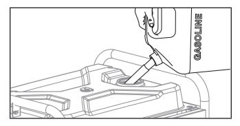
5. Screw on the gasoline cap and wipe away any spilled fuel.
