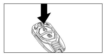
6. Push and hold the programming button approximately three seconds until the red light turns off.
