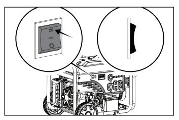
2. Turn the battery switch to the "ON" position.
