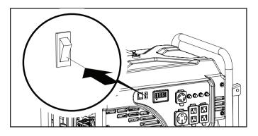
Push and hold the wireless set button found on the side of the control panel for approximately three seconds until the red light turns on.
