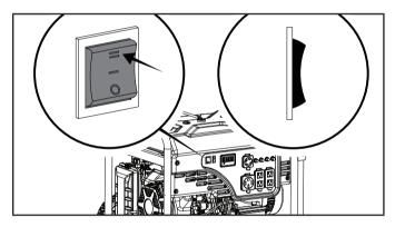
Press and release the START button on the remote control. DO NOT hold the button down, only press the button once. The engine will attempt to start six times.
