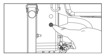
Push and release the STOP <sup>™</sup> button on the remote key fob. The red light blinks once to erase the remote program.
