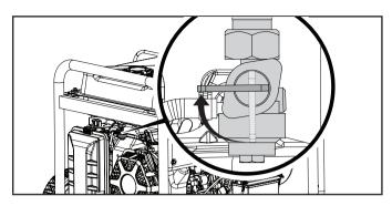
**Important:** Always ensure that the fuel valve, the ignition switch, and the battery switch are in the "OFF" position when the generator will not be used for an extended period of time.
