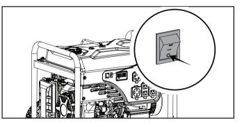
4. *If generator was started electrically,* press the battery switch to the "OFF" position.
