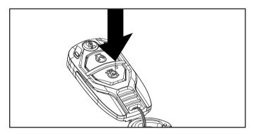
Push and release the START Subtract button on the remote key fob. The red light blinks once to program the remote.
