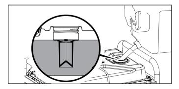
The approximate fuel level is shown on the fuel gauge on top of the fuel tank.
