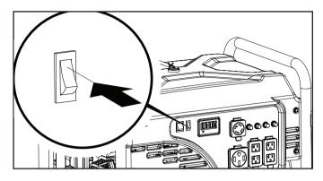
2. Press and hold the ignition switch to the "START" position. Release as the engine begins to start. If the engine fails to start within five seconds, release the switch and wait at least ten seconds before attempting to start the engine again.
