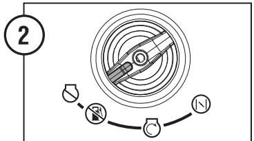
**NOTE:** This unit has a **GASOLINE OFF** setting that can be used before storing the unit for long periods of time. Refer to the user manual for details.
