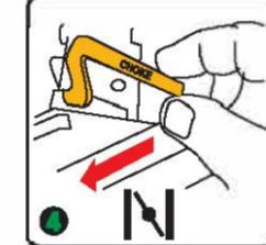
Move choke lever located on engine to START position
