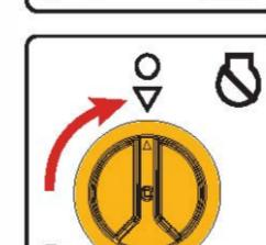
Turn the fuel selector switch to OFF (O)position
