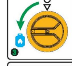
Turn the fuel selector switch to LPG position
