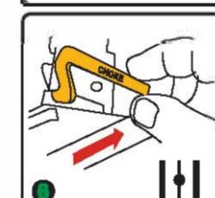
Move choke lever to RUN Position
