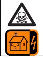
Improper connections to a building electrical system can allow electrical current from the generator to back feed into the utility lines. Such back feed may electrocute utility company workers or others who contact the lines during a power outage, and the generator may explode, burn or cause fires when utility power is restored. Consult the utility company or a qualified electrician.
