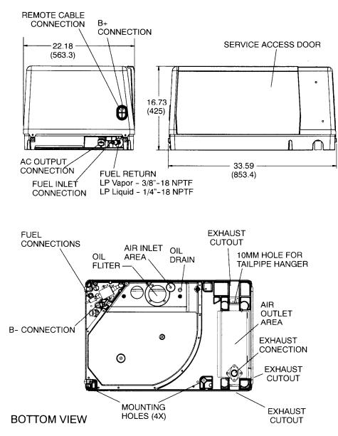
**Note:** This outline drawing is provided for general reference only and is not intended for design or installation. For more information see Operation and Installation manuals or obtain 500-3234 drawing and wiring diagram from your distributor/dealer.
