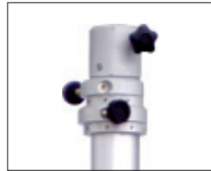
2) Place on the mast head and fasten by the relevant hand-wheel, the floodlight unit.
