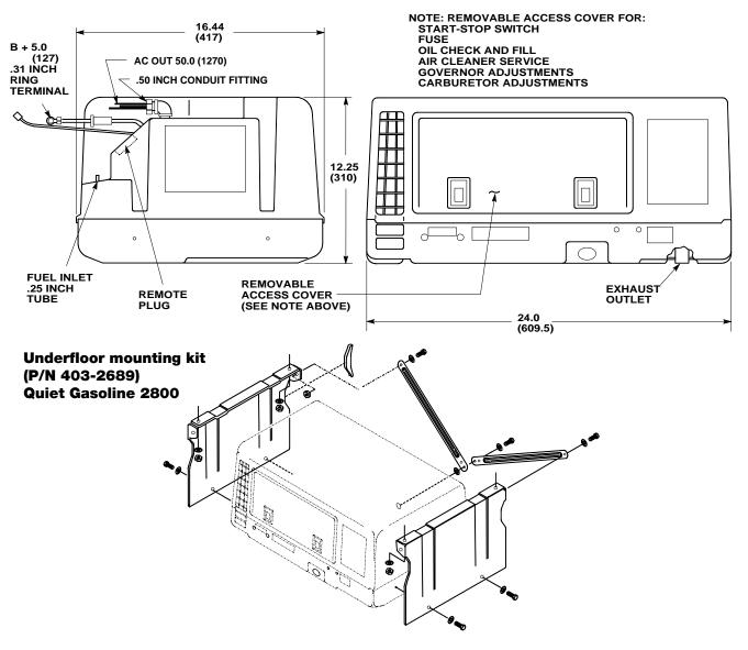
**Note:** This outline drawing is provided for general reference only and is not intended for design or installation. For more information see Operation and Installation manuals or obtain 500-2182 drawing and wiring diagram from your distributor/dealer.
