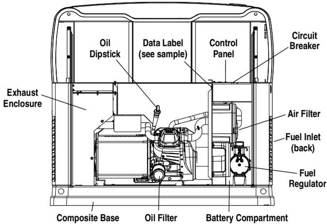
Figure 1.2 – 10kW, V-twin, GT-530 Engine (door removed)
