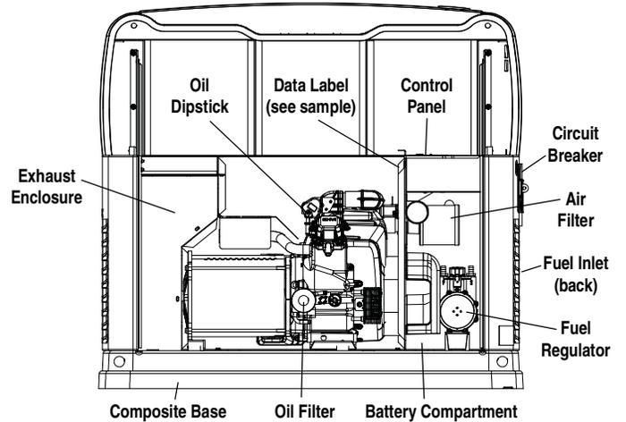
Figure 1.3 – 13, 14, 16, 17 and 20kW, V-twin, GT-990/GT-999 Engine (door removed)
