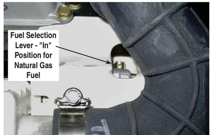
**Figure 1.6 - 10kW, GT-530 (Inlet Hose Slid Back)**
