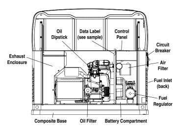
Figure 1.3 – 12, 14, 16, 17 and 20kW, V-twin, GT-990/GT-999 Engine (door removed)
