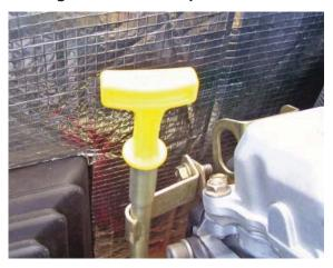
Figure 4.3 — Oil Dipstick and Fill, 12, 14, 16, 17 & 20kW
