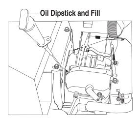
Figure 4.2 — Oil Dipstick, 10kW
