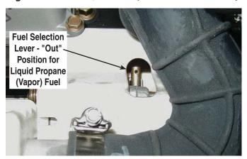
Figure 1.7 - 12, 14, 16, 17, & 20kW, GT-990/GT-999 (Airbox Cover Removed)
