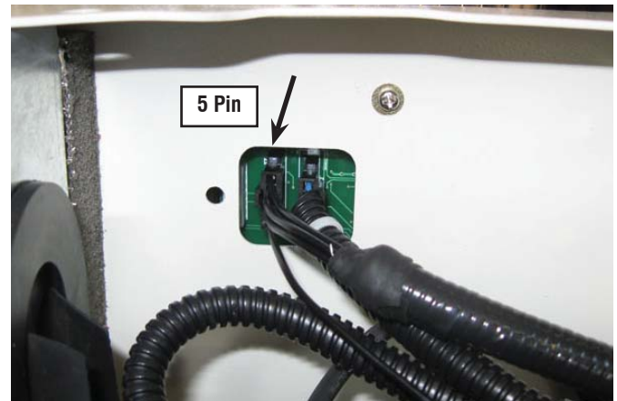
Figure 6 – Plug in the 5-pin plug
