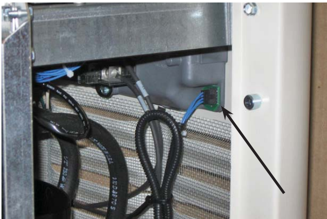
Figure 4 – Unplug the existing 4-pin plug
