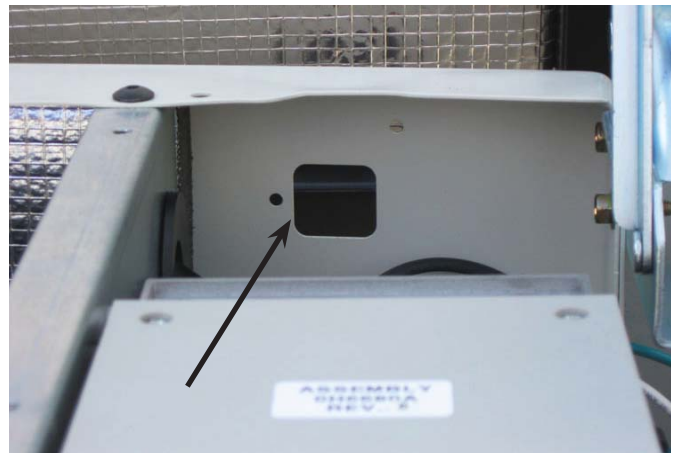
Figure 2 — Remove Cover Plate & Rubber Gasket
