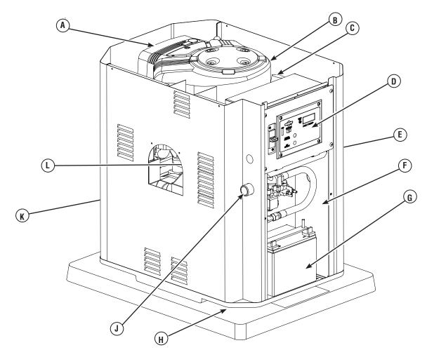
Generator is shown with roof, plastic access cover and control panel cover removed for clarity.
