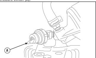
The oil pressure switch uses normally closed contacts that are held open by engine oil pressure during operation. Should oil pressure drop below the 8 psi range, switch contacts close and the engine is shut down.
