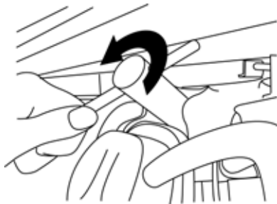
FIGURE 36: Spark Plug Removal
