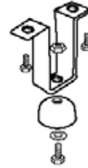
FIGURE 4: Rubber Stopper Attachment to Support Leg
