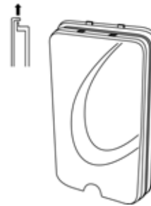
FIGURE 31: Air Cleaner Cover—Release Tabs
