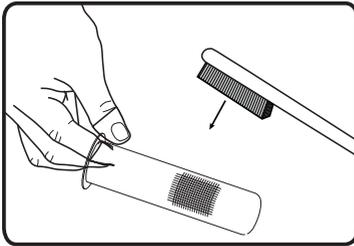
4. Replace the spark arrester if it is damaged.
