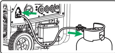
**NOTE:** Do not place LPG cylinder in the path of muffler outlet.
