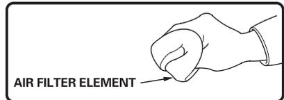
(c) Lastly, put the element in the case and install it securely.
