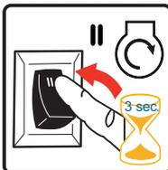
**REMINDER: MUST HAVE SOLID RED INDICATOR LIGHT TO BE ABLE TO START THE GENERATOR. THE GENERATOR CANNOT BE STARTED DURING BATTERY POWER SAVING MODE UNLESS THE FUEL SELECTOR SWITCH IS TURNED TO THE "OFF" POSITION AND THEN TURNED BACK TO THE "GAS" POSITION. See Indicator light-Battery power Saving Mode section for more information.**
