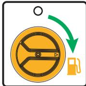
**NOTE:** When the fuel selector switch is turned to the "GAS" position, the indicator light will become **RED** up to **4 minutes** (before goes off). Starting the engine successfully during these **4 minutes** will turn the indicator light **GREEN**.
