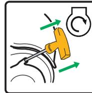
If the engine fails to start in 1-2 pulls with choke in the "RUN" position, then move choke lever to "START" position and repeat the "PULL-TO-PRIME" step.
