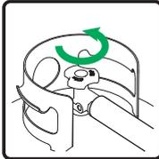
5. Turn the fuel selector switch to "LPG" position.
