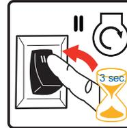
**REMINDER:** MUST HAVE **SOLID RED INDICATOR LIGHT** TO BE ABLE TO START THE GENERATOR. THE GENERATOR CANNOT BE STARTED DURING **BATTERY POWER SAVING MODE** UNLESS THE FUEL SELECTOR SWITCH IS TURNED TO THE "OFF" POSITION AND THEN TURNED BACK TO THE "LPG" POSITION.
