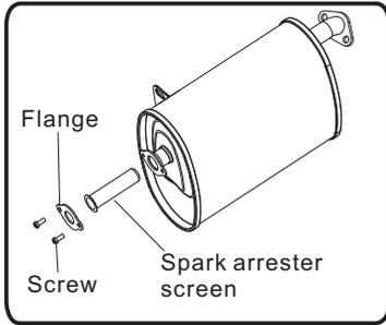
3. Carefully remove the carbon deposits from the spark arrester screen with a wire brush.
