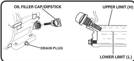
4. Using oil funnel, slowly pour contents of provided oil bottle into oil fill opening to the "H" mark on dipstick. Be careful do not overfill. Overfilling with oil could cause the engine to not start or hard starting.
