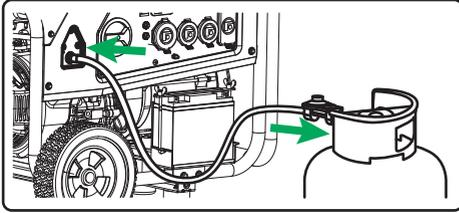
**NOTE:** Do not place the LPG cylinder in the path of muffler outlet.
