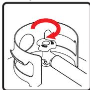
4. Turn the fuel selector switch to "GAS" position.
