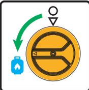
**NOTE:** When the fuel selector switch is turned to the "LPG" position, the indicator light will become **RED** up to **4 minutes**(before goes off). Starting the engine successfully during these **4 minutes** will turn the indicator light **GREEN**.
