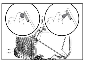
5. Replace the spark arrestor and spark arrestor screen if it they damaged.
