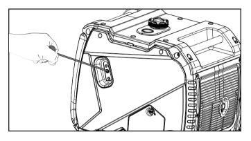
Do not over-choke. As soon as engine starts, push the choke button one time to set the choke to the "RUN" position. Choke button will no longer be illuminated when in "RUN" position.
