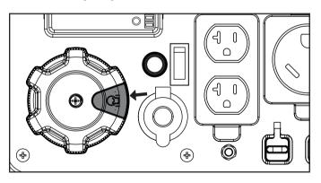
6. Do not over-choke. As soon as engine starts, push the choke button one time to set the choke to the "RUN" position. Choke button will no longer be illuminated when in "RUN" position.
