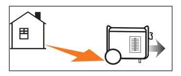
If misused and operated in an unapproved and unsafe location that results in the accumulation of poisonous CO gas inside an enclosed or partially enclosed space, for example a house, garage or a garage with the door partially open, CO Shield<sup>®</sup> will automatically shut off the generator and then will illuminate a blinking red LED light. **Read the action label for next steps.**
