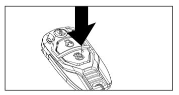
Push and release the START Subtract button on the remote key fob. The blue LED on wireless set button will blink once to indcate the remote has been programmed.
