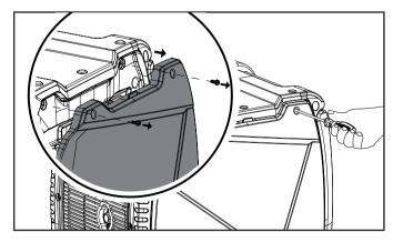
2. Locate the air filter plastic cover and remove by pinching the clips together and pulling the cover off.
