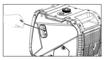
6. Do not over-choke. As soon as engine starts, move the choke lever to the "RUN" (left) position.
