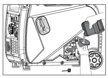
5. Check engine oil level before each use and add as needed.
