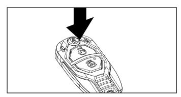
Push and hold the wireless set button approximately three seconds until the blue LED on wireless set button turns off.
