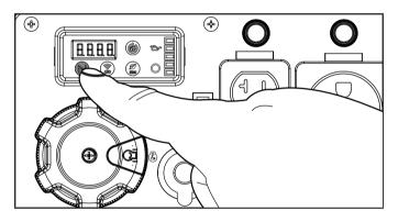
5. Press and hold the yellow ignition switch on the EZ Start Dial toward the center of the dial. Release as the engine begins to start. If the engine fails to start within five seconds, release the switch and wait at least ten seconds before attempting to start the engine again.
