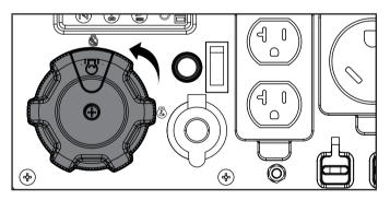
4. *If battery switch is in the "ON" position,* press the battery switch to the "OFF" position.
