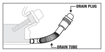
4. Ensure the oil drain hose is lower than the engine and allow the oil to drain completely into an appropriate container.
