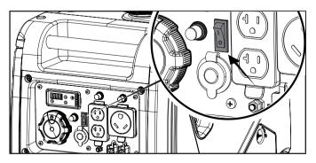
**Important:** Always ensure that the EZ Start Dial and battery switch are in the "OFF" position when the generator will not be used for an extended period of time.
