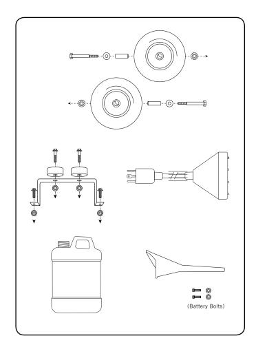
Your generator requires some assembly. This unit ships from our factory without oil. It must be properly serviced with fuel and oil before operation.
