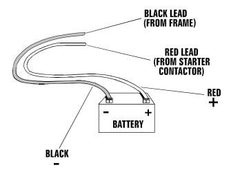
Figure 6.3 – Battery Cable Connections
