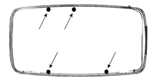
Figure 4.2 — Mounting Hole Location
