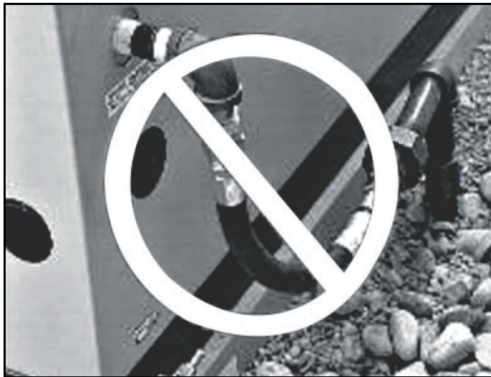
Figure 5-4. Incorrect Routing of Flexible Hose
